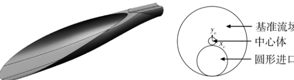
图 8 进气道进口截面及无黏气动构型 Fig. 8 Schematic of intake plane and inviscid configuration
